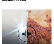
Stainless steel has the property of not rusting. However, if tools made out of conventional steel are used for stainless steel components or screws, the particles left behind from these tools can adhere to the surface and then rust. This effect known as extraneous rust - can impair the visual appearance and even cause structural damage that may result in expensive repair work. The wear particles that cause this rust effect can be prevented by using stainless steel tools.
