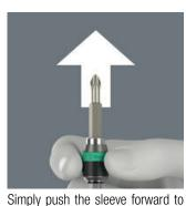
change the bit. The spring mechanism lifts the bit off the magnet and unlocks the tool. The bit can be easily removed. The rapid-out function makes it easy to remove even the smallest bits without extra tools.
