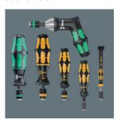
Wera torque screwdrivers. With a factory pre-set torque value set to the smallest scale value. For all applications, where the same constant torque and repeat accuracy are required. The torque can be changed with an extra tool within the measuring range (recalibration kit can be ordered with the code number 05137003001). Afterwards you can check the set value using an off-the-shelf torque tester.
