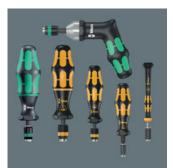
Wera torque screwdrivers. With a factory pre-set torque value set to the smallest scale value. For all applications, where the same constant torque and repeat accuracy are required. The torque can be changed with an extra tool within the measuring range (recalibration kit can be ordered with the code number 05137001001). Afterwards you can check the set value using an off-the-shelf torque tester.
