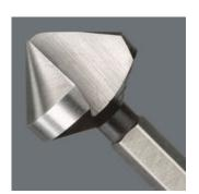
1-flute countersink bits, 90°Application: Deburring, chamfering and countersinking1/4" drive suitable for holders as per DIN 3126-D 6.3 (ISO 1173)Hexagon shaft for very high torque transfer1 tipGuaranteed vibrationfree and scratch-free operationOptimal countersink surface qualityLong service lifePerfect chip removalHigh corrosion protection
