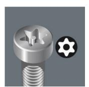
TORX® tools with a borehole prevent the unauthorised unfastening of safety screws. The screws contain a pin that protrudes into the drive profile so that "normal" TORX® tools cannot be used. This pin fits into the borehole of TORX® BO tools allowing safety screws to be unfastened.
