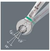
Thanks to the open end side offset by 7.5°, double hexagon geometry and an adjusted application method (placement - screwdriving - turning - replacement - screwdriving - turning, etc), even screwdriving challenges allowing a return angle of less than 30° can be solved.
