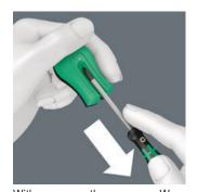
With the Wera magnetiser/demagnetiser: simply run the tool down the positive side of the Wera magnetiser/demagnetiser and the tool immediately becomes magnetised and is able to hold the screw securely on the blade.
