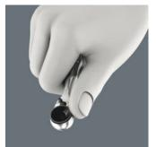
High working speeds can be attained with the Zyklop Mini bit ratchet. The thumb wheel is important, enabling more rapid screwdriving, and the lever of the Zyklop Mini only needs to be used for the final tightening of the screw.
