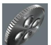
The fine tooth mechanism, with its 60 teeth, allows a small return angle of only 6° - ideal for precision work.
