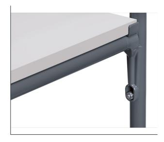
These electrically conductive struts in slate grey are easily screwed under an existing shelf. That stabilises the upper structure and increases the capacity of the inserted shelves. The shelf located on top of the longitudinal connector struts has a carrying capacity of 110kg instead of 50kg due to the support. The electrical conductivity is maintained. 1 pair per ESD-trolley is included.
