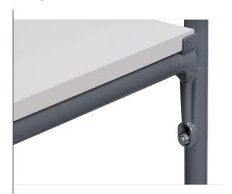
These electrically conductive struts in slate grey are easily screwed under an existing shelf. That stabilises the upper structure and increases the capacity of the inserted shelves. The shelf located on top of the longitudinal connector struts has a carrying capacity of 110kg instead of 50kg due to the support. The electrical conductivity is maintained. 1 pair per ESD-trolley is included.
