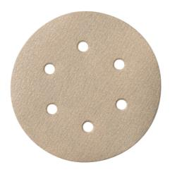
25 Hook and loop sanding sheets, 150 mm, P 80, "paint", "professional" series for paints, lacquers, and filler compounds, for random orbital sanders, aluminium oxide, stearate-coated
