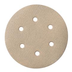
25 Hook and loop sanding sheets, 150 mm, P 100, fpaint, "professional" series for paints, lacquers, and filler compounds, for random orbital sanders, aluminium oxide, stearate-coated
