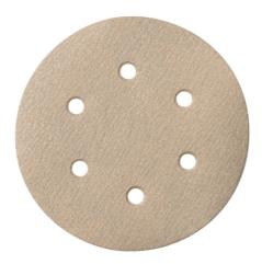
25 Hook and loop sanding sheets, 150 mm, P 120, "paint", "professional" series for paints, lacquers, and filler compounds, for random orbital sanders, aluminium oxide, stearate-coated
