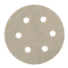
25 Hook and loop sanding sheets, 80 mm, P 180, paint, "professional" series for paints, lacquers, and filler compounds, for random orbital sanders, aluminium oxide, stearate-coated
