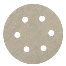
25 Hook and loop sanding sheets, 80 mm, P 240, "paint", "professional" series for paints, lacquers, and filler compounds, for random orbital sanders, aluminium oxide, stearate-coated
