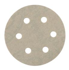
25 Hook and loop sanding sheets, 80 mm, P 320, "paint", "professional" series for paints, lacquers, and filler compounds, for random orbital sanders, aluminium oxide, stearate-coated
