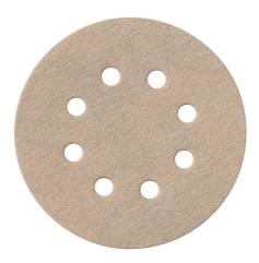
25 Hook and loop sanding sheets, 125 mm, P 80, "professional" series for paints, lacquers, and filler compounds, for disc sanders, aluminium oxide, stearate-coated
