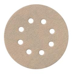
25 Hook and loop sanding sheets, 125 mm, P 240, "professional" series for paints, lacquers, and filler compounds, for disc sanders, aluminium oxide, stearate-coated
