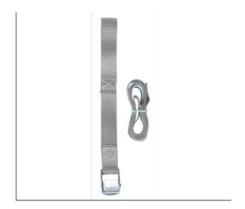
Two pieced. By flat loops 100 mm long on both ends very easy to fasten in any position at the truck frame. Tight end 0,3 m with aluminium belt clamp, lose end 2,5 m. Due to the asymmetric parting suitable for small and largetransport goods.
