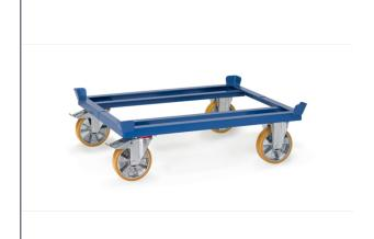
For pallets and boxes. Sturdy sectional steel construction with 4 catch corners for stacking, powder coated. 2 swivel and 2 fixed- wheels 200 x 50 mm. Swivel castors with wheel lock, according to the European Standard EN 1757-3 (safety of platform trolleys). Polyurethane wheels, hubs with ball bearings. Low low rolling resistance, smooth running, no road noise. Optional extras are only delivered in a set with pallet dollies because they are welded together.
