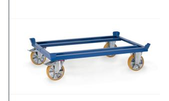
For pallets and boxes. Sturdy sectional steel construction with 4 catch corners for stacking, powder coated. 2 swivel and 2 fixed- wheels 200 x 50 mm. Swivel castors with wheel lock, according to the European Standard EN 1757-3 (safety of platform trolleys). Polyurethane wheels, hubs with ball bearings. Low low rolling resistance, smooth running, no road noise. Optional extras are only delivered in a set with pallet dollies because they are welded together.
