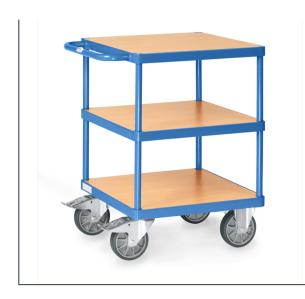
Modular system: Tubular steel and sectional steel, welded and powder coated blue RAL 5007, surface durably protected, resistant to impact and scratches. 2 shelves made of derived timber material boards, surface beech grain. 2 swivel and 2 fixed-wheel castors, TPE tyres, hubs with groove ball bearing. Swivel castors with wheel locks, according to the European Standard EN 1757-3 (safety of platform trolleys). Capacity upper and middle shelf 200 kg.
