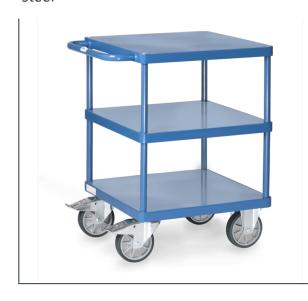
Modular system: Tubular steel and sectional steel, welded and powder coated, surface durably protected, resistant to impact and scratches. 2 Square platforms made of steel sheet, flush with frame, powder coated. 2 swivel and 2 fixed-wheel castors, TPE tyres, hubs with groove ball bearing. Swivel castors with wheel locks, according to the European Standard EN 1757-3 (safety of platform trolleys). Capacity upper shelf 200 kg.
