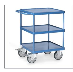
Modular system: Tubular steel and sectional steel, welded and powder coated, surface durably protected, resistant to impact and scratches. 2 square platforms, trays made of steel sheet, with rim 10 mm high, welded oil-tight, powder coated. 2 swivel and 2 fixed-wheel castors, TPE tyres, hubs with groove ball bearing. Swivel castors with wheel locks, according to the European Standard EN 1757-3 (safety of platform trolleys). Capacity upper shelf 200 kg.
