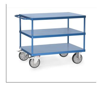
Modular system: Tubular steel and sectional steel, welded and powder coated, surface durably protected, resistant to impact and scratches. 3 platforms made of steel sheet, flush with frame, powder coated. 2 swivel and 2 fixed-wheel castors, TPE tyres, hubs with groove ball bearing. Swivel castors with wheel locks, according to the European Standard EN 1757-3 (safety of platform trolleys). Capacity upper and middle shelf 200 kg.
