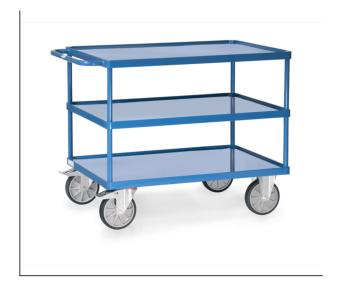
Modular system: Tubular steel and sectional steel, welded and powder coated, surface durably protected, resistant to impact and scratches. 3 platforms, trays made of steel sheet, with rim 10 mm high, welded oil-tight, powder coated. 2 swivel and 2 fixed-wheel castors, TPE tyres, hubs with groove ball bearing. Swivel castors with wheel locks, according to the European Standard EN 1757-3 (safety of platform trolleys). Capacity upper and middle shelf 200 kg.
