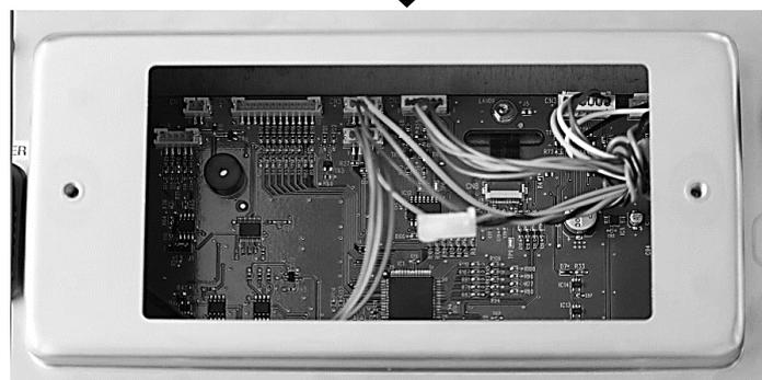
3. Carefully detach the back of the terminal from the front.
