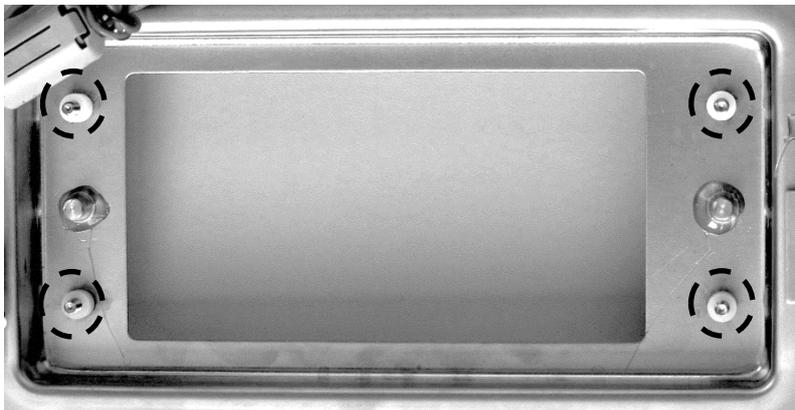
7. Place the relay output with the holes on the screw pins
