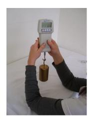
5. This position is held until "F" appears on the display. Then the weight can be removed and the adjustment is completed. However, if "E" appears on the display - repeat steps 1. to 5. until "F" confirms successful adjustment.
