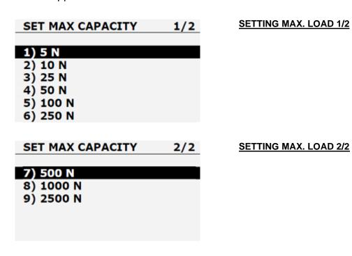
4. Use the UP and DOWN arrow keys to select the maximum load, press the selected value and hold for a moment.
