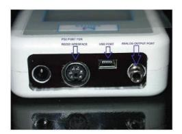
There is an analog output on the device. This generates a signal that goes from +2V to -2V. This signal is a percentage of the maximum value of the force gauge. FOR EXAMPLE..: FL100 50N is measured in the direction of pull, then a -1V signal is applied to the analog output. 75N in compression direction, then + 1.5V is present at the analog output. If the instrument is in PASS - Fail mode, 2V for PASS and 0V for FAIL are present at the analog output.
