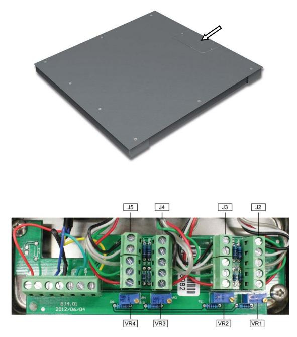
Adjustment of weighing cell J2 takes place at the potentiometer VR1. Adjustment of weighing cell J3 takes place at the potentiometer VR2. Adjustment of weighing cell J4 takes place at the potentiometer VR3. Adjustment of weighing cell J5 takes place at the potentiometer VR4. Increase the value turning to the right, reduce the value turning to the left.
