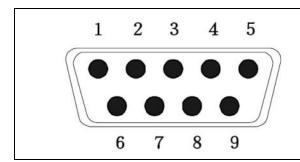
Pin 2: TXD - output Pin 3: RXD - input Pin 5: GND - signal ground
