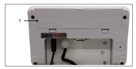
Open the battery compartment cover (1) at the base of the display unit and insert the rechargeable battery. Charge the battery for at least 12 hours before initial use.
