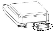
2. Insert the batteries / rechargeable batteries into the battery holder:  $4\ x\ 1.5\ V\ AA$
