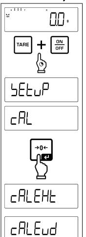
⇒ Press and hold the TARE and ON/OFF buttons simultaneously to enter the setup menu.
