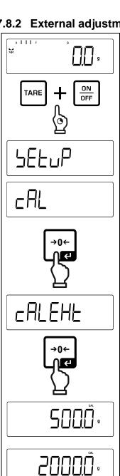
⇒ Press and hold the TARE and ON/OFF buttons simultaneously to enter the setup menu.
