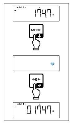
The unit for quick selection can be determined when the **[MODE]**-button is shortly pressed for the first time.
