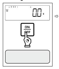
Keep **ON/OFF** button pressed until the display disappears
