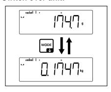
⇒ Using **[MODE]** button, it is possible to switch over between the enabled unit 1 and unit 2.
