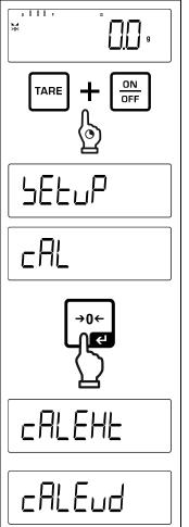
⇒ Press and hold the TARE and ON/OFF buttons simultaneously to enter the setup menu.
