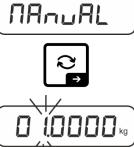
⇒ Using the navigation keys ↓↑ select the setting Select < ☐☐□☐☐L > and confirm by pressing the → button.
