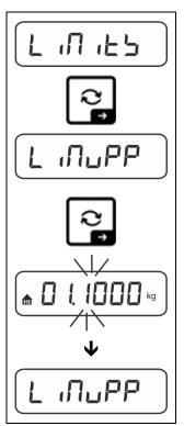
⇒ Using the navigation keys ↓↑ select the setting Select < └ ╷ ☐ , └ └ └ > and confirm on → button.
