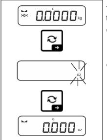
The unit for quick selection can be determined when the -button is shortly pressed for the first time.
