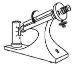
Close the cover, turn on the polarimeter and wait until the sodium vapour lamp has warmed up (approx. 10 minutes).
