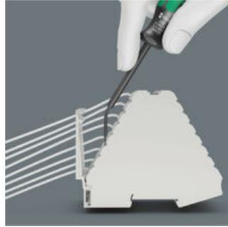
Terminal blocks hold the wire ends mechanically. The force required for this is applied by a spring in the case of tension spring terminals. The spring must be opened by a tool in order to be able to insert the wire ends. The special actuation tools from Wera allow operating the tension spring terminals - even in tight spaces such as switch cabinets. The curved blade also allows spring terminals to be reached where straight-blade tools cannot be used.
