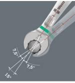
Thanks to the open end side offset by 7.5°, double hexagon geometry and an adjusted application method (placement - screwdriving - turning - replacement screwdriving - turning, etc), even screwdriving challenges allowing a return angle of less than 30° can be solved.
