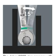
The Joker 6003 ring spanner with its special open end geometry open end offset by 7.5° and the double hexagon profile - doubles the placement possibilities when repeatedly turning the wrench 180° around the longitudinal axis. Bolts and screw heads can be "accessed" every 15°. The Joker 6003 will automatically find the respective placement point after every turn.
