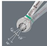
Thanks to the 7.5° offset open end, the double hexagon geometry and an improved application method (placement - screwdriving - rotation - re-placement - screwdriving - rotation etc), even screwdriving situations that have a return angle of less than 30° can be solved.
