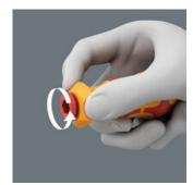
The ratchet mechanism also allows fast "spinning" while screwdriving.
