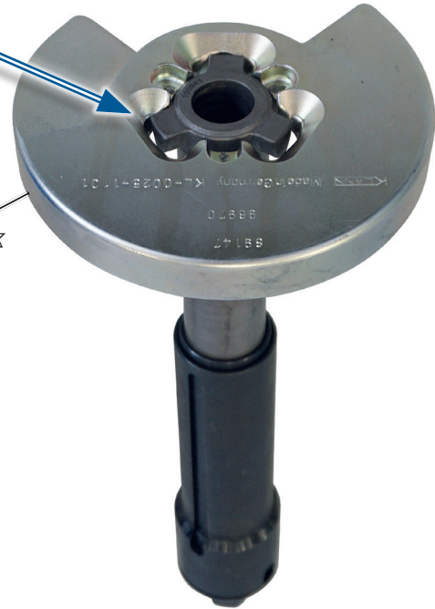
Upper spring plate with three-point safety lock
