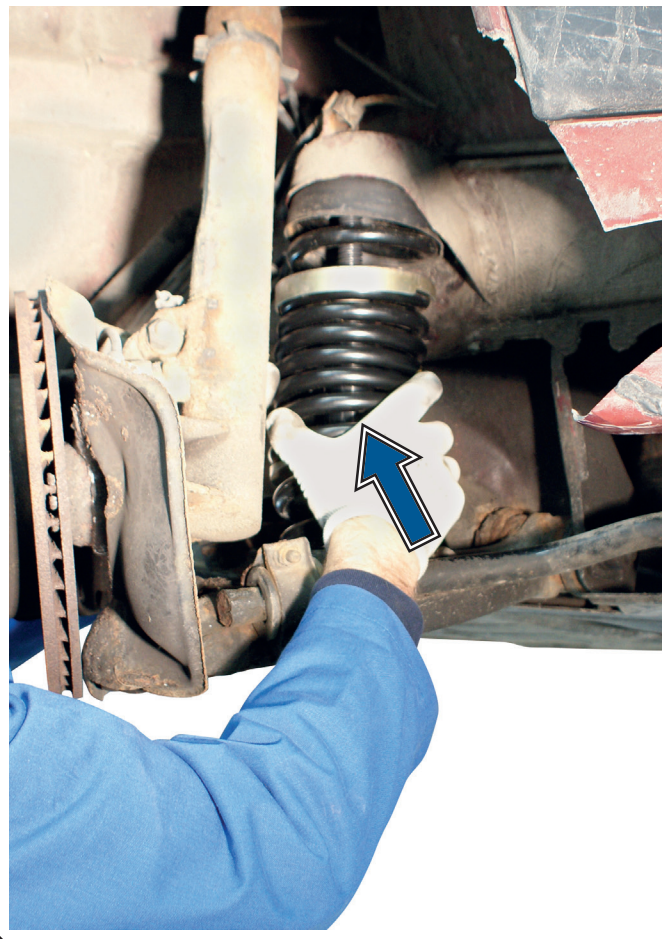
📸 15: Insert the compressed spring into the axle.
