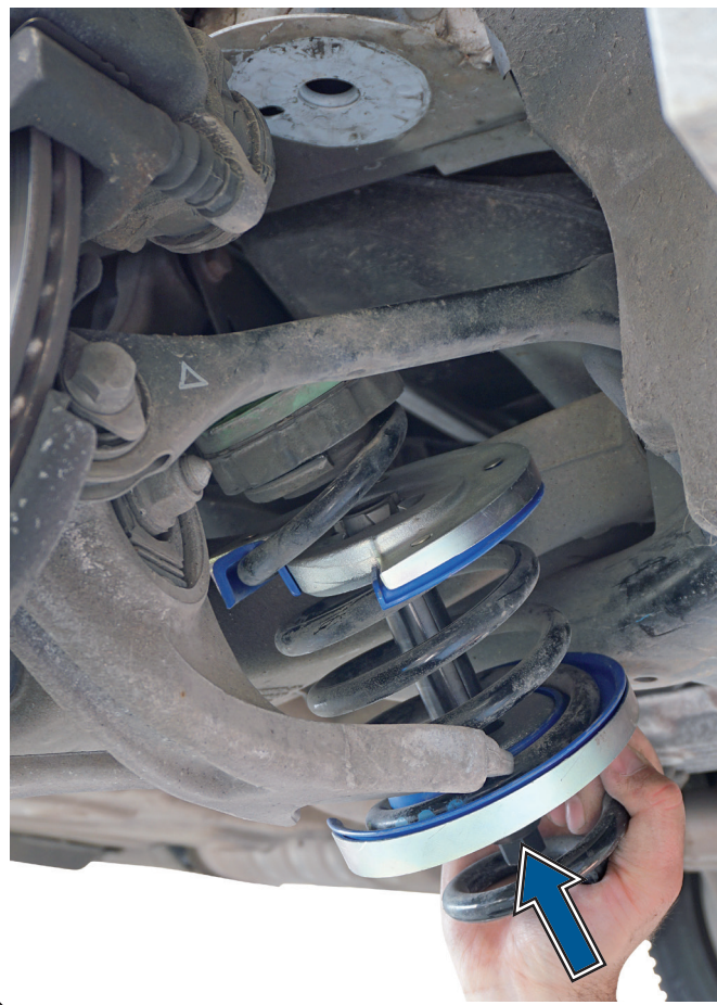
📸 17: Insert the compressed spring into the axle.
