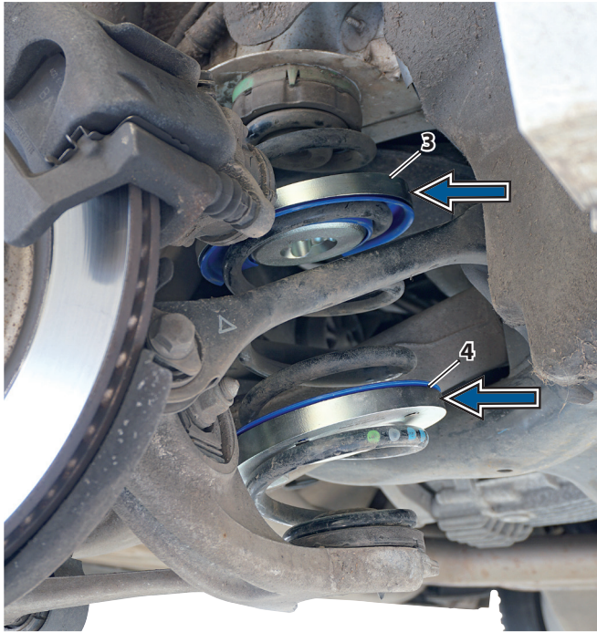
📷6: Insert the pressure plates "3 + 4" into the spring.
