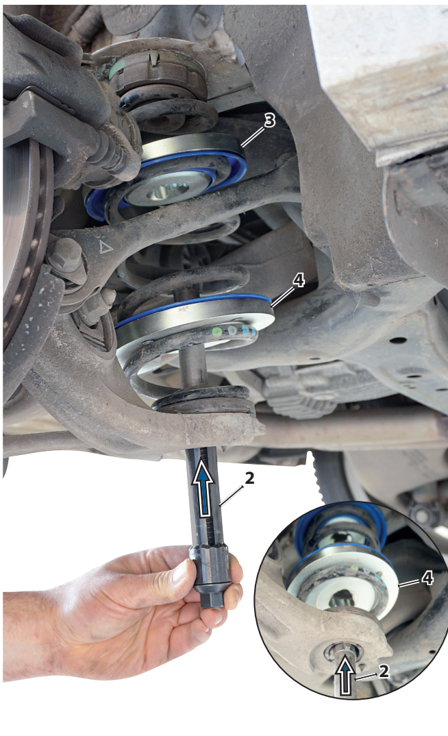
📷7: Insert the compressor cylinder "2" and lock it.
