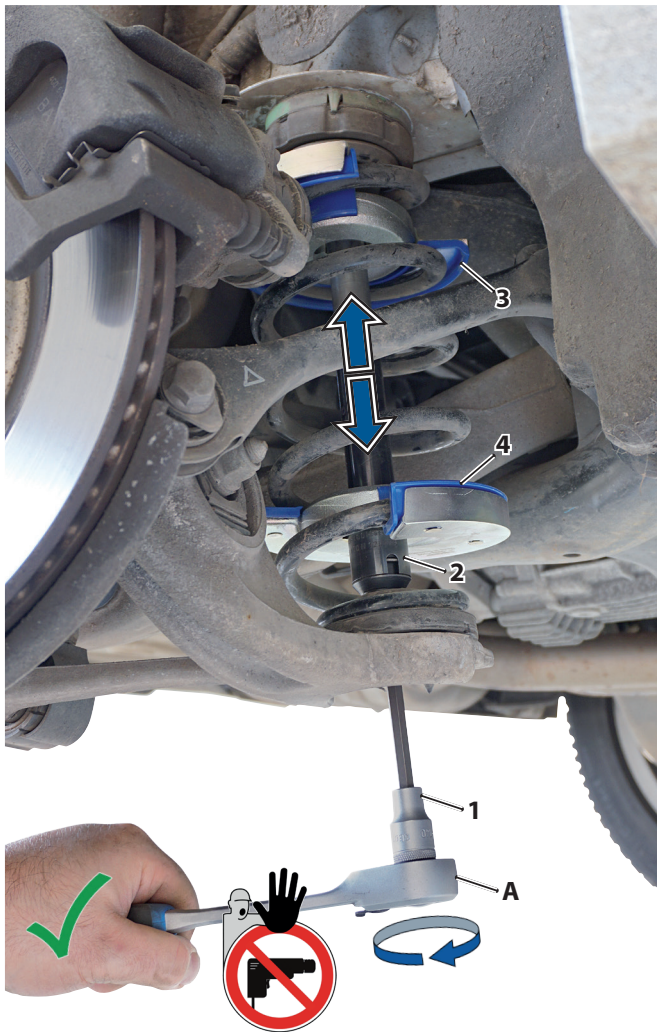
📷 18: Release the internal-type spring compressor.
