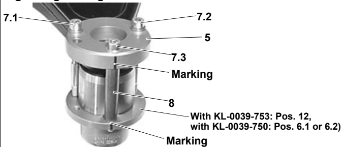
Fig. 8: Applying the press frame against wishbone, removing the suspension ball joint.
