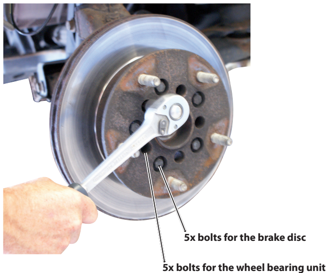
📷 17: Screwing cheese-head screws [A4] into steering knuckles.
