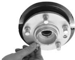
Fig. 5: Mounting the tool to steering knuckle/stub axle.
