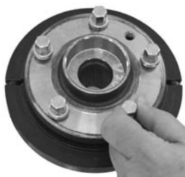
Fig. 9: Mount tool. Install wheel hub bearing unit
