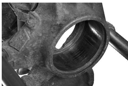
Fig. 21: Clean wheel bearing bore.
