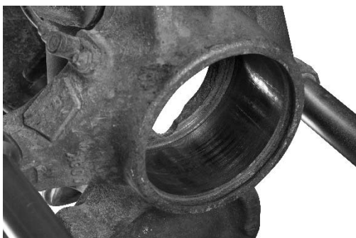
Fig. 41: Clean wheel bearing bore.
