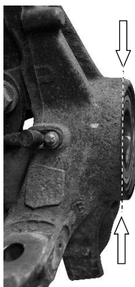
Fig. 46: Safety ring is fully engaged in the groove.
