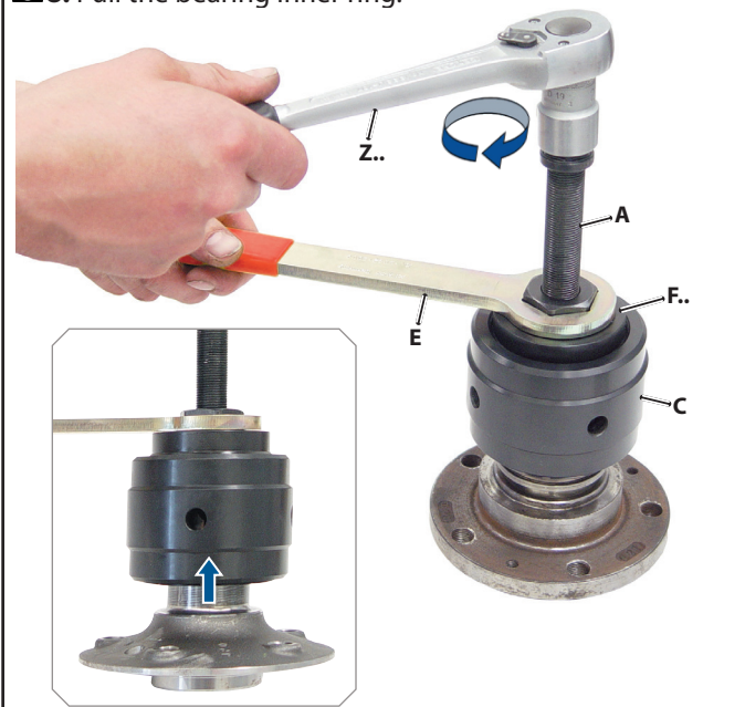
📸8: Pull the bearing inner ring.
